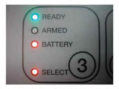
Figure 4-12 Verify the green READY Lights are on steady
