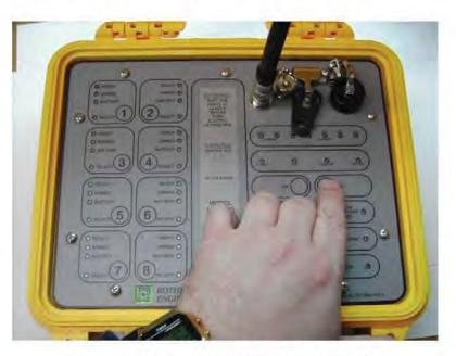
Figure 4-14 Turn the Controller Unit OFF
