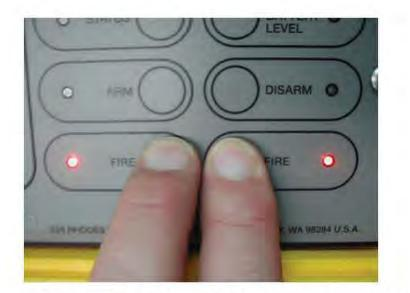
Figure 4-11 Firing the ARMED and SELECTED Remote Units
