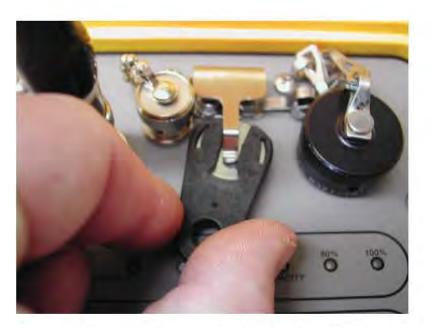
Figure 4-15 Remove the Controller's Key
