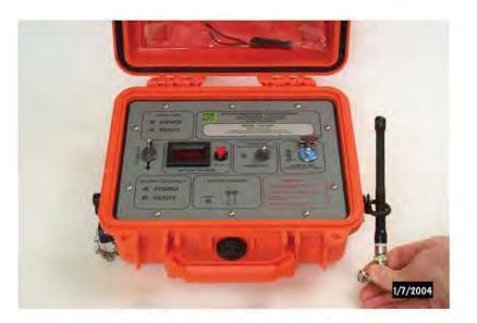
Figure 4-2 Remote Antenna Installation
