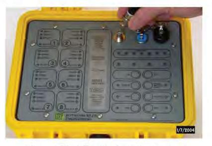
Figure 4-1 Installing the Controller Antenna
