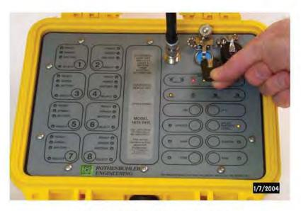
Figure 4-6 Inserting the Controller KEY
