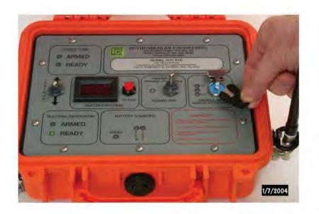
4.1.12. Install the enable key into the Remote Unit and observe the yellow light next to the ENABLE KEY begins flashing. If the Controller is in Safety Poll® mode, this light will turn on steady within 15 seconds to show that full 2-way communications are working.
